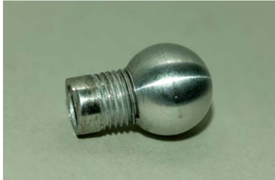
Fig. 11: Cementing cap with a screwed on load attachment.
