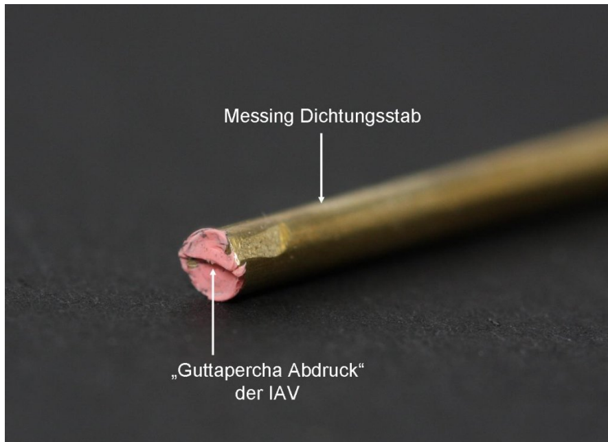
Fig. 22: Brass sealing rod with „gutta-percha“- casting of the IAC. The rod serves as a sealant of the IAC and liquid entrance to the IAC.
