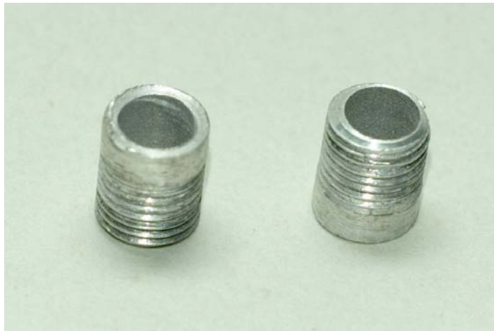
Fig. 7: Cementing caps from aluminum.
