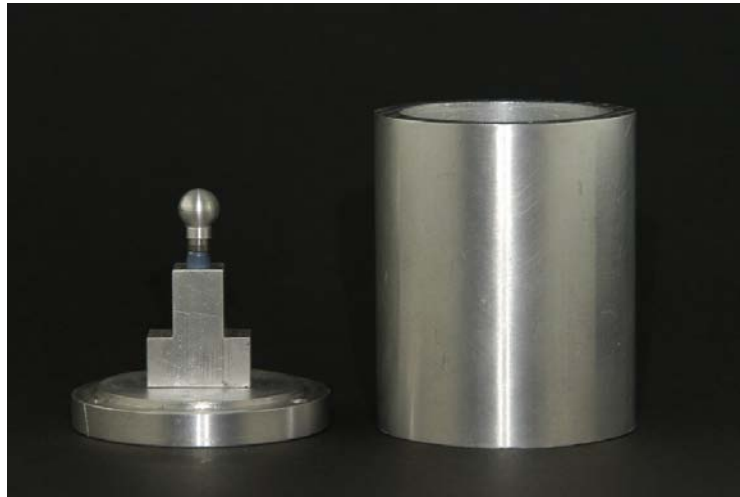
Fig. 13: Embedding form with T1 and implant.
