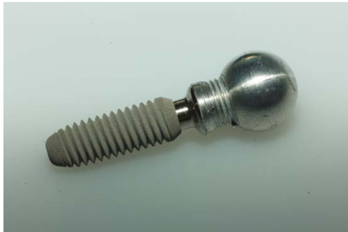
Fig. 16: Implant with cemented cap and load attachment (ball).
