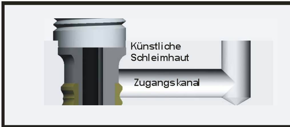
Fig. 21: Schematic arrangement of the IAC, the artificial mucous membrane and the entrance channel to the IAC.
